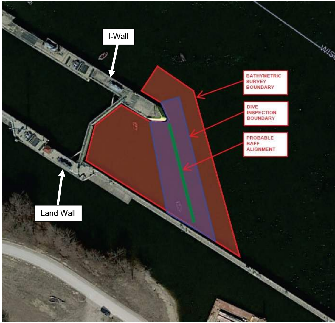
Figure 1 - Inspection Area Map
